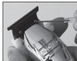
**Step 5** – Once the blade is adjusted to zero gap or your liking, gently tighten the two screws on each side of the blade while holding the zero gap tool in place. If the blade is not adjusted to satisfaction after testing, repeat the adjusting process.
