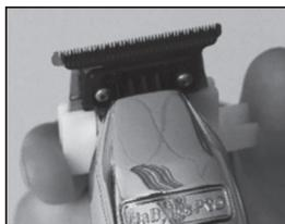
**Step 3** – Using your fingers on each side of the zero gap tool, push up until the black cutting blade is even with “or” slightly below the fixed blade.
